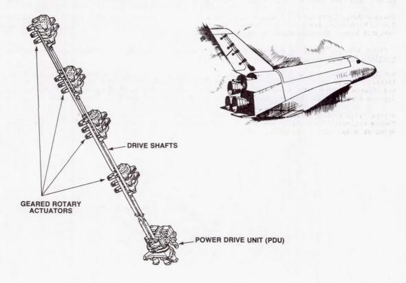
Figure 1 Rudder/Speed Brake Actuation System The Power Drive Unit (PDU) responds to electrical command signals that operate electrohydraulic servovalves. The servovalve operation ports hydraulic pressure to hydraulic motors which in turn provide rotary power to PDU gearbox. The PDU is presented schematically in Figure 2.
