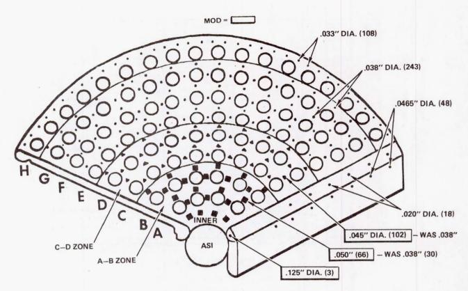
Figure 19. Fuel Preburner Injector Modification.
