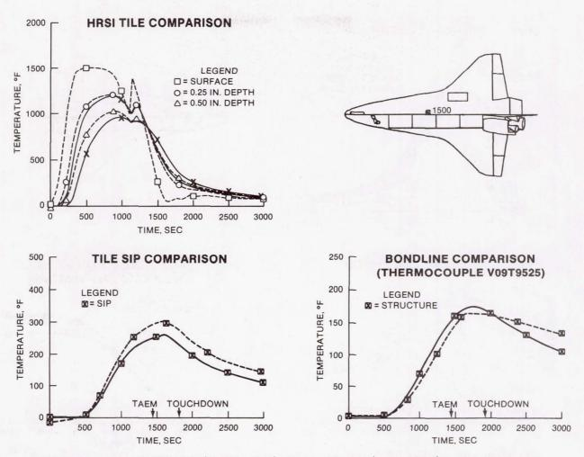
FIGURE 12.- STS-5 FLIGHT DATA (DASHED LINES) VERSUS ANALYSES (SOLID LINES): BODY POINT 1500.
