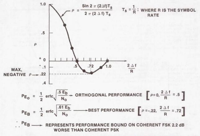
FIGURE 20.- P VERSUS FREQUENCY DEVIATION FOR CONTINUOUS-PHASE FM DIGITAL MODULATION.
