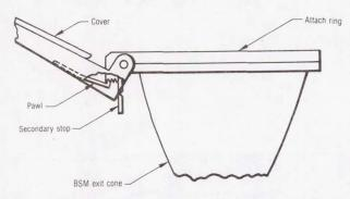
Figure 8. Open Cover Immediately Before Secondary Stop Engagement.
