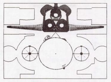
Figure 3. ORBITER/BIPOD CLEARANCE DURING MATING
