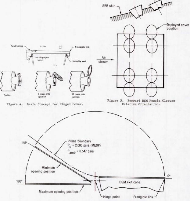
Figure 6. Forward BSM Nozzle Closure Allowable Opening Angles.
