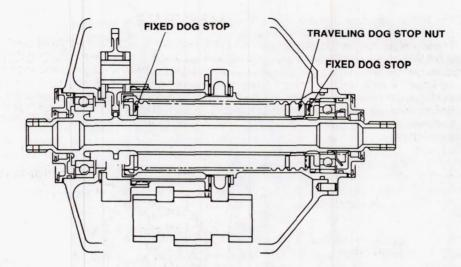
Figure 3 Stops Located on Inboard Actuator
