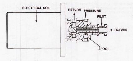
Figure 12 Spool and Sleeve Solenoid Valve 3-Way, 2-Position
