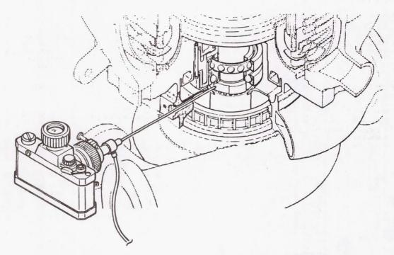
Figure 26. HPOTP No. 3 Bearing Photographic Condition Recording.
