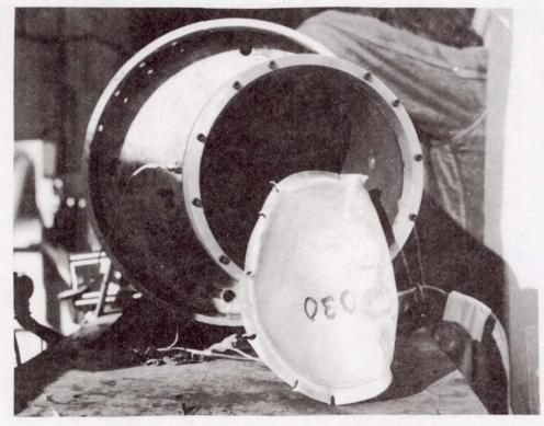
Figure 15. Aft Mounted BSM Nozzle Closure - Post-Test.
