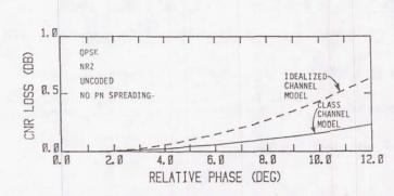
Figure 2b. COMPARISON OF PARAMETER SENSITIVITIES FOR CLASS CHANNEL MODEL AND IDEALIZED CHANNEL MODEL FOR MODULATOR PHASE ERROR.
