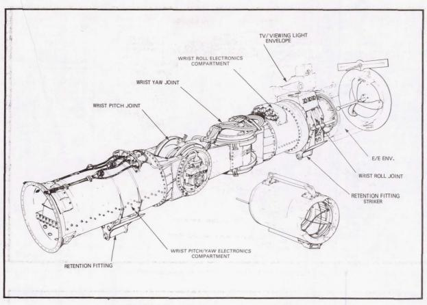
Figure 8 Overall Configuration of the Wrist Joint
