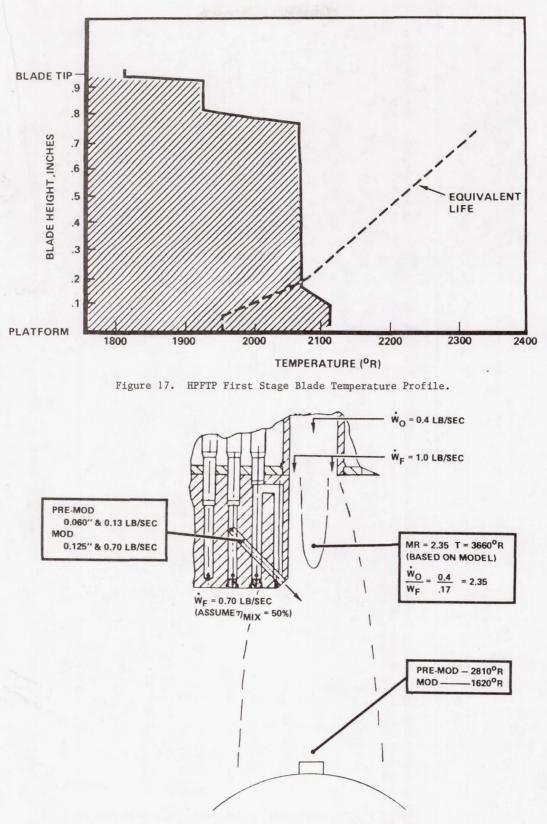
Figure 18. Fuel Preburner Baffle Modification (ASI Core Temp.).
