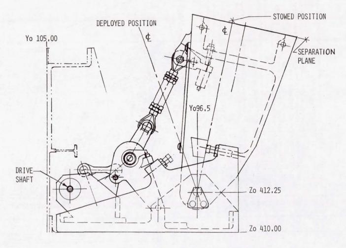
Figure 6. Retention Support - Stowed and Deployed Positions
