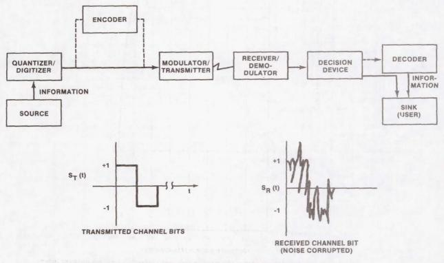
FIGURE 6.- FUNCTIONAL BLOCK DIAGRAM OF A DIGITAL COMMUNICATION CHANNEL.
