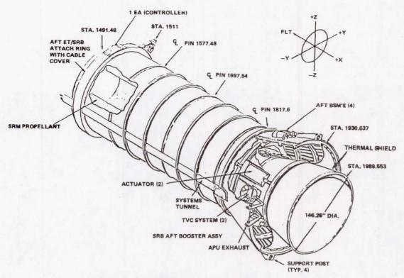
Figure 2. SRB TVC Subsystem and Actuators.
