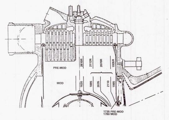
Figure 20. Fuel Preburner Temperature Comparisons Radial Distribution.
