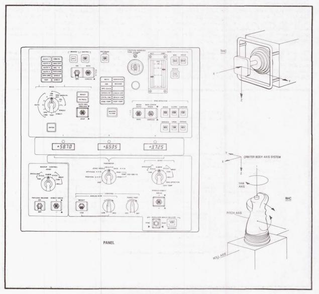
Figure 2 Display and Control Panel, and Hand Controllers
