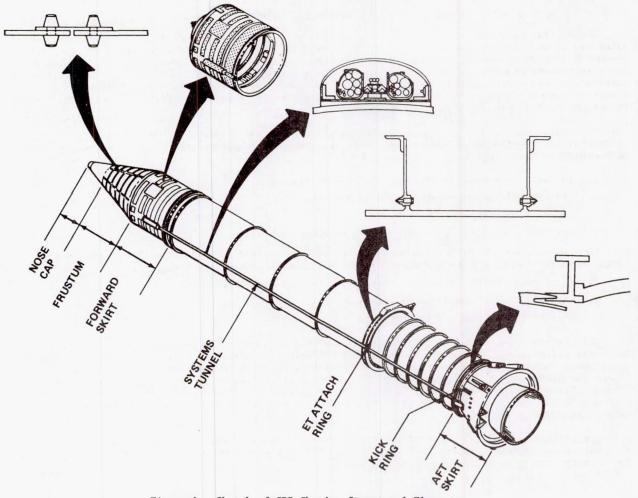
Figure 1. Sketch of SRB Showing Structural Elements.
