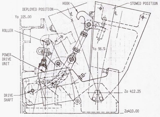
Figure 5. Shoulder Support - Stowed and Deployed Positions
