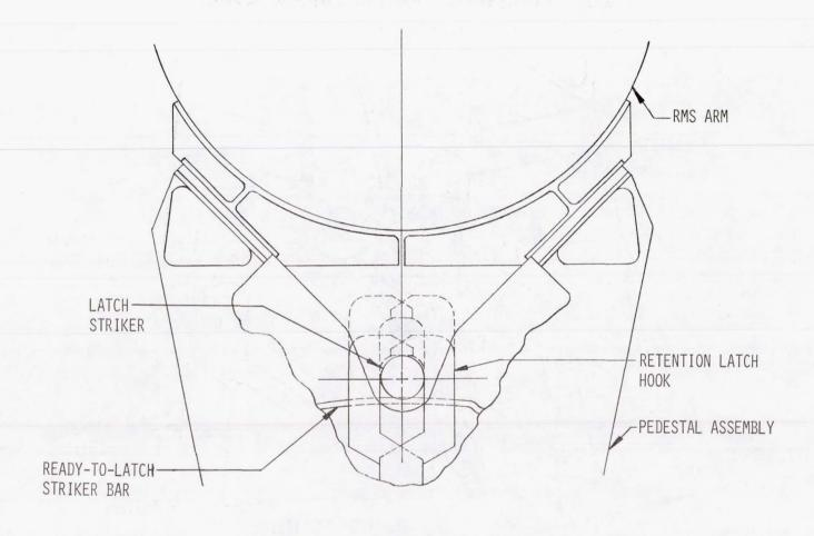
Figure 7. Manipulator Positioning Mechanism Latch and Unlatch Capabilities of RMS ARM
