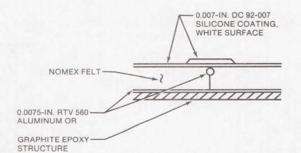
FIGURE 5.- FRSI TPS INSTALLATION.
