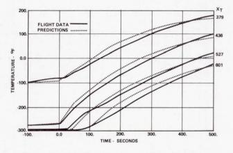
Figure 6. LO2 Tank Structural Temperatures.
