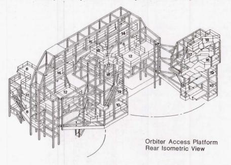
Split into two hinged sections, the overall size of each is 17 feet x 20 feet x 50 feet, high. Platforms 10, 16 and 19 swing up and down and service the engines and parts of the fin. They operate using hydraulic actuators and also telescope horizontally.
