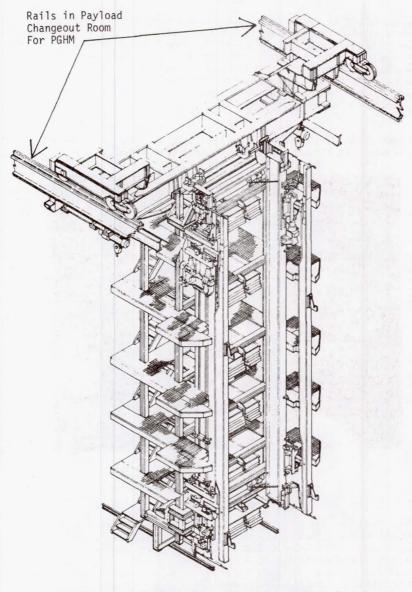
FIGURE 11. PAYLOAD GROUND HANDLING MECHANISM (PGHM)
