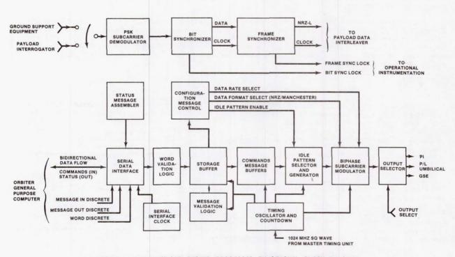
FIGURE 5.- NASA PAYLOAD SIGNAL PROCESSOR FUNCTIONAL BLOCK DIAGRAM.
