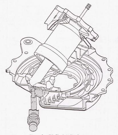
Figure 9. SRB GN<sub>2</sub> Spin Nozzle.
