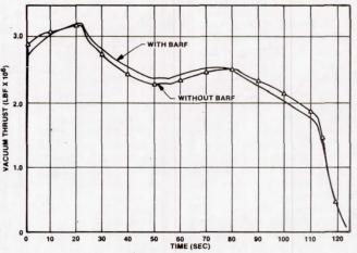
FIGURE 3. EFFECT OF BARF ON TC-227A-75 THRUST PERFORMANCE
