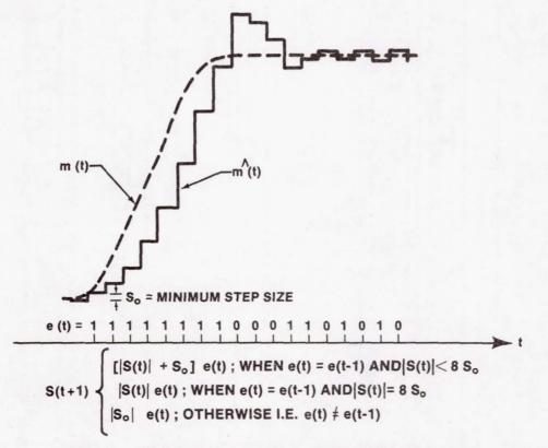
FIGURE 4.- MODIFIED ABATE ADAPTIVE DELTA MODULATION ALGORITHM.
