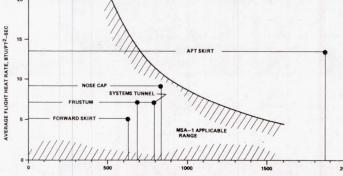
TOTAL FLIGHT HEAT LOAD, BTU/FT<sup>2</sup> Figure 5. SRB Elements TPS Thermal Requirements Compared with the Thermal Capability of MSA-1.
