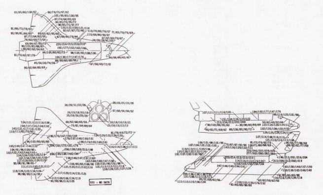
FIGURE 15.- STRUCTURAL TEMPERATURE RISE (OF) RESULTING FROM ENTRY HEATING: STS-1 TO STS-5.
