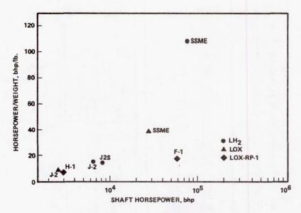
Figure 7. Turbopump Power/Weight Experience.
