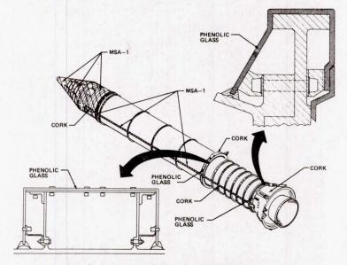
Figure 6. Sketch of SRB Showing TPS Utilized.
