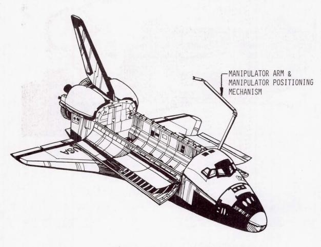
Figure 1. RMS ARM On Its On-Orbit Use Position
