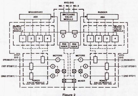
Figure 2 Power Drive Unit Schematic
