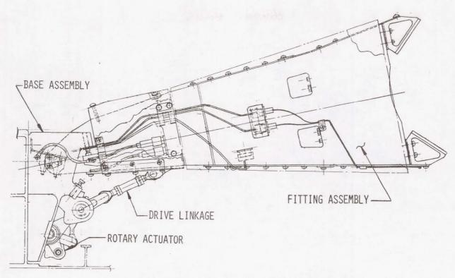
Figure 3. Manipulator Positioning Mechanism Pedestal Assembly
