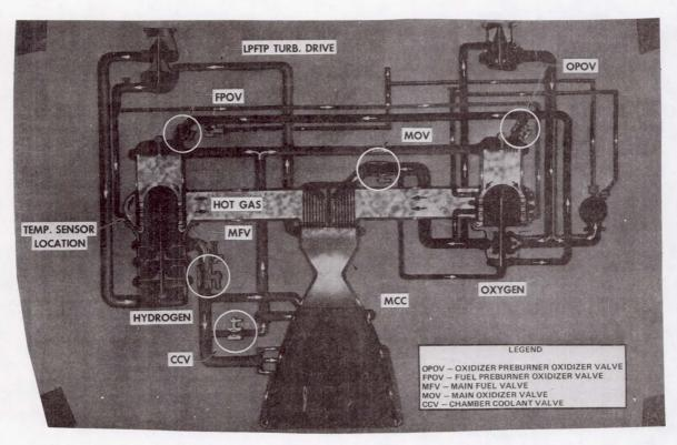
Figure 10. SSME Propellant Flow Schematic.
