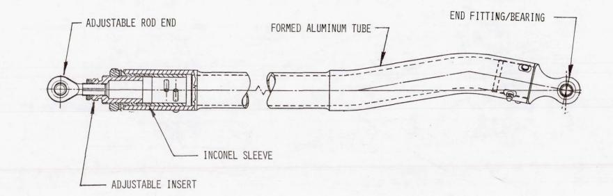
FIGURE 4. CURVED ALUMINUM LINK ASSEMBLY
