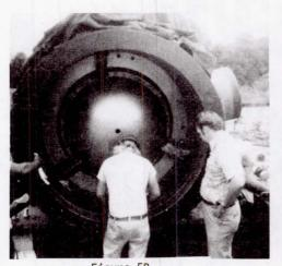
Figure 5B Top Hemispherical Bearing Assembled Inside Housing
