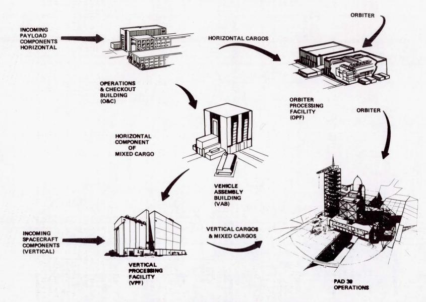
FIGURE 1. PAYLOAD TRANSPORTATION FLOW AT KSC
