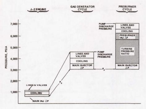
Figure 5. Rocket Engine Pressure Schedule.
