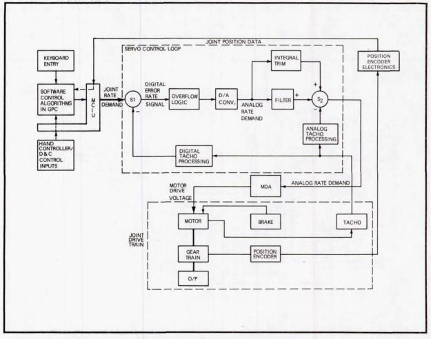
Figure 4 System Block Diagrm - Typical Joint
