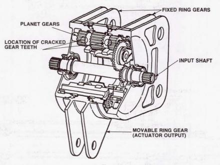
Figure 5 Geared Rotary Actuator
