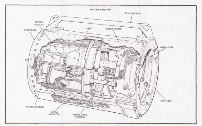
Figure 9 End Effector Arrangement
