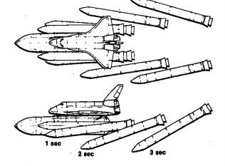
Figure 2. Computer Simulation of SRB Separation Sequence.
