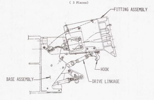
Figure 4. Manipulator Positioning Mechanism Shoulder Assembly
