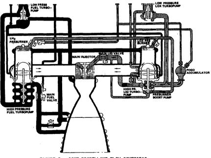
FIGURE 8. SSME PROPELLANT FLOW SCHEMATIC
