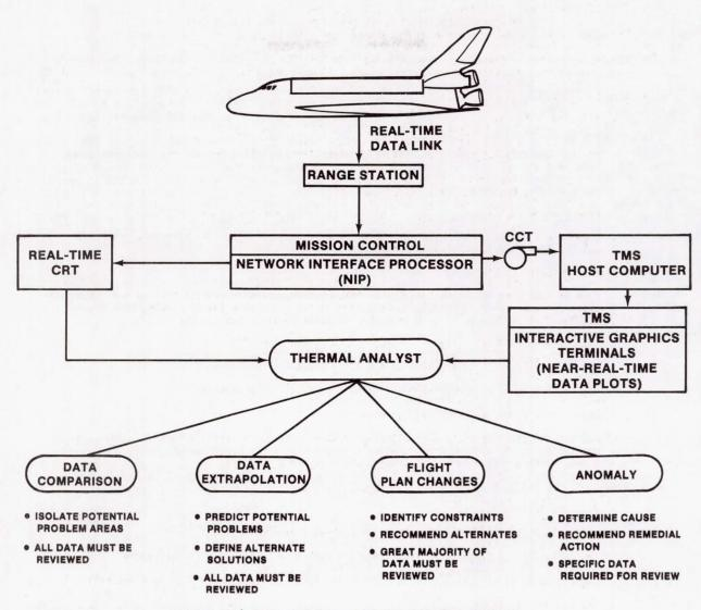
FIGURE 11.- REAL-TIME DATA FLOW AND ANALYSIS SCHEMATIC.
