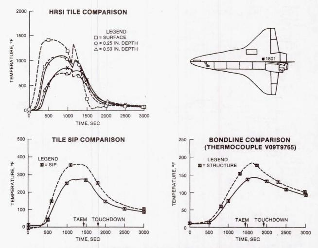
FIGURE 13.- STS-5 FLIGHT DATA (DASHED LINES) VERSUS ANALYSES (SOLID LINES): BODY POINT 1801.
