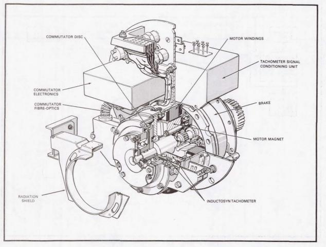
Figure 5 Motor Module Configuration
