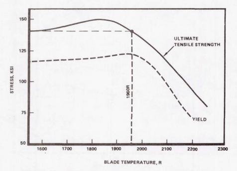
Figure 14. HPFTP Turbine Blade Metal Temperature (MM-246-DS).
