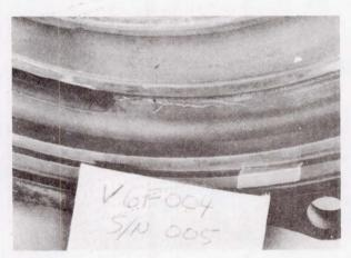
FIGURE 24.- CRACK AT 25° VENT, APU EXHAUST HOUS-ING.
