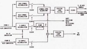
FIGURE 4: OVERVIEW OF SSRE, INTEGRATED CARRIER LOOP/SYMBOL SYNC
