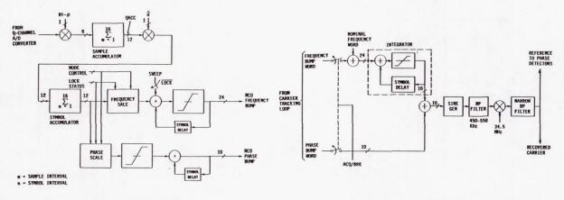
FIGURE 5: CARRIER TRACKING LOOP
