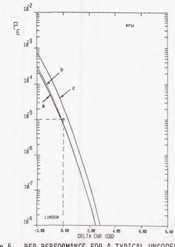
BER PERFORMANCE FOR A TYPICAL UNCODED Figure 5. TDRSS RETURN LINK. (A) UNSCRAMBLED, 50% TRANSITION DENSITY; (B) UNSCRAMBLED, 10% TRANSITION DENSITY; (C) SCRAMBLED.
