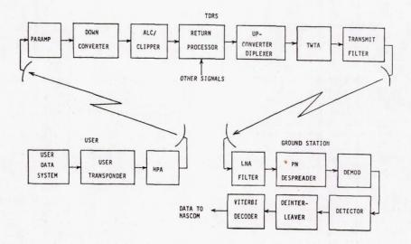
Figure 1. TYPICAL LINK MODEL.
