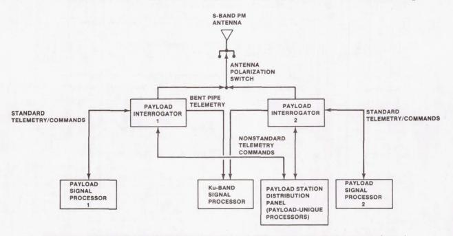
FIGURE 2.- ORBITER PAYLOAD S-BAND COMMUNICATIONS SYSTEM FUNCTIONAL CONFIGURATION (FINAL).
