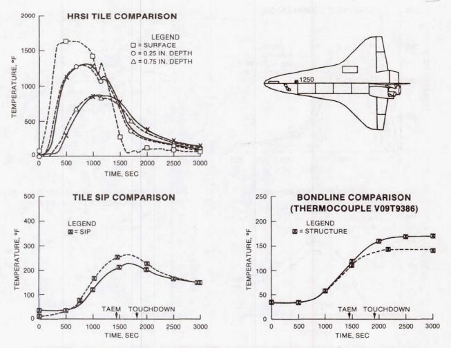
FIGURE 11.- STS-5 FLIGHT DATA (DASHED LINES) VERSUS ANALYSES (SOLID LINES): BODY POINT 1250.
