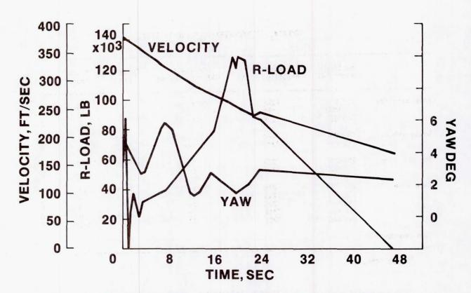
FIGURE 2.- TYPICAL LOAD/TIME PROFILE: 240 000-POUND VEHICLE WEIGHT, DELAYED PITCHOVER, 20-KNOT CROSSWIND.
