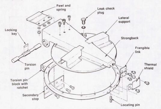
Figure 7. Exploded View of Forward BSM Nozzle Closure.
