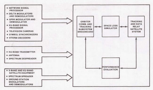
FIGURE 6. - ORBITER COMMUNICATIONS AND TRACKING SUBSYSTEM BREADBOARD SOURCES.
