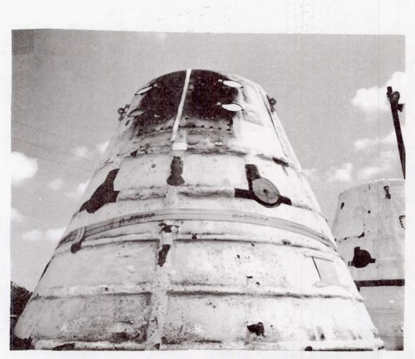
Figure 12. BSM Hinged Covers on Nose Cone of Recovered Shuttle Booster After Flight.
