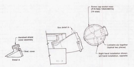
Figure 9. Hinged Cover Assembled to BSM Exit Cone.
