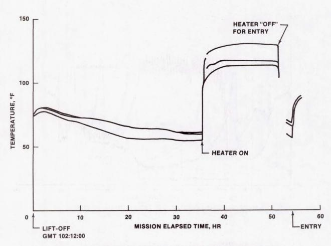
FIGURE 18.- STS-1 FORWARD RCS COMPARTMENT PORT HEATER PANEL TEMPERATURE PROFILE.
