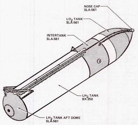
Figure 1. Initial ET TPS Configuration.
