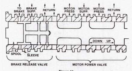
Figure 11 Modified Control Valve Moving From Null to Up Position
