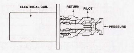
Figure 13 Poppet Solenoid Valve, 3-Way, 2-Position
