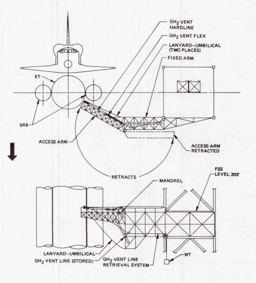
FIGURE 3. GH 2 VENT CONCEPT III (BASE FROM FSS)
