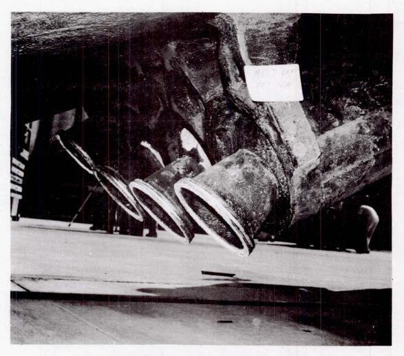
Figure 16. Aft Mounted BSMs After Recovery From Flight.
