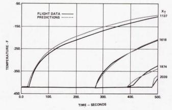
Figure 7. LH2 Tank Structural Temperatures.
