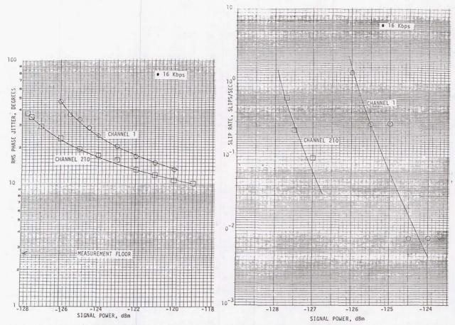
Figure 2.3. Shuttle PSP-PI Subcarrier Loop Phase Jitter Performance.
