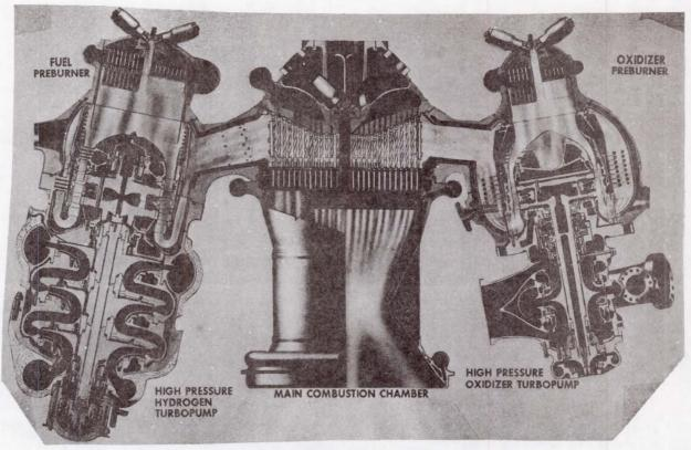
Figure 11. SSME Powerhead Component Arrangement.
