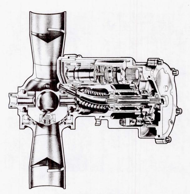
FIGURE 9.- A/C MOTOR VALVE CROSS SECTION.
