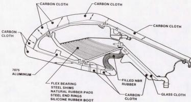
FIGURE 8. NOZZLE FORWARD ASSEMBLY
