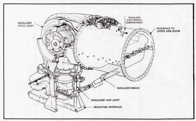
Figure 6 Overall Configuration of the Shoulder Joint
