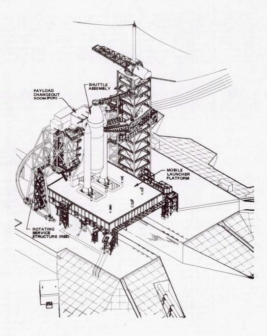
FIGURE 1. PAYLOAD CHANGEOUT ROOM WITH PGHM AND ACCESS STANDS
