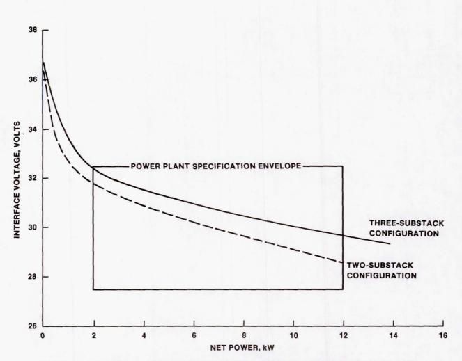
FIGURE 5.- COMPARISON OF PERFORMANCE DATA FOR TWO-SUBSTACK AND THREE-SUBSTACK POWERPLANTS.
