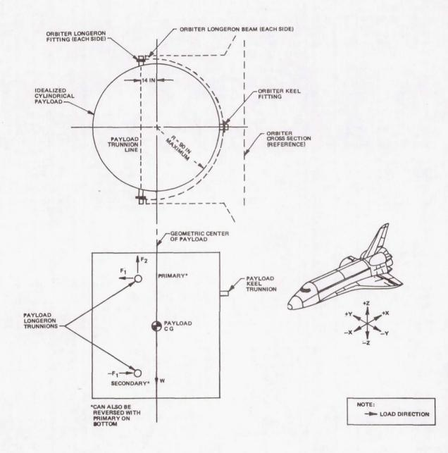
FIGURE 3. PAYLOAD TRUNNION FORCES
