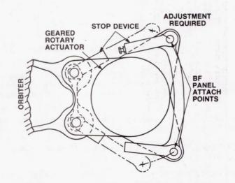
Figure 2 Stops Located on Actuator Output
