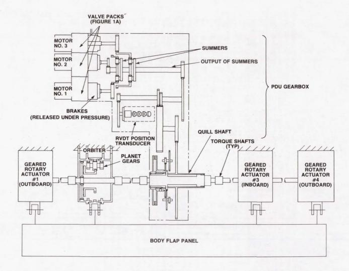
Figure 1 Body Flap Actuation Subsystem
