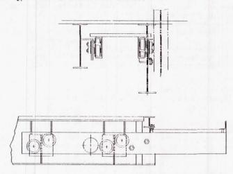
Manually operated hoists are also used for lighter swing-up and down platforms. These are of a simple-geared winch type with removable hand cranks.
