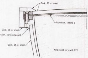
Figure 13. Aft Mounted BSM Nozzle Closure Configuration (After Proof Test).
