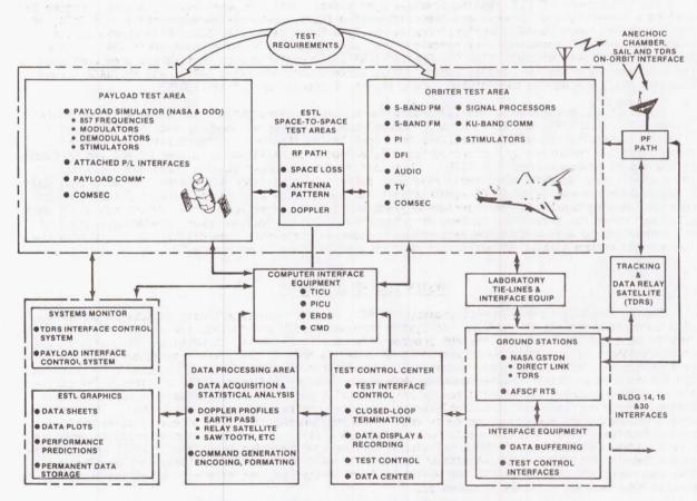
FIGURE 14.- ESTL PAYLOAD TEST CONFIGURATION.
