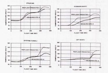
Figure 11. Typical SRB Structural Temperature Responses when Protected with MSA-1.
