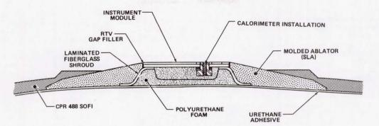
Figure 5. Hardened Instrumentation Island.
