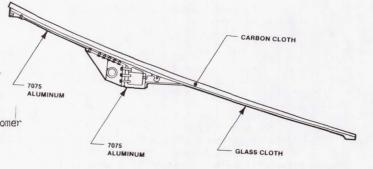
FIGURE 9. NOZZLE EXIT CONE ASSEMBLY
