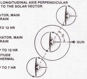
BETA ANGLE ( $\beta$ ) = ANGLE BETWEEN SOLAR VECTOR AND ORBIT PLANE
