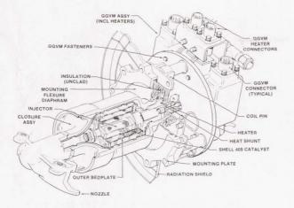
FIGURE 13.- MIN-MOD GAS GENERATOR - BASELINE.
