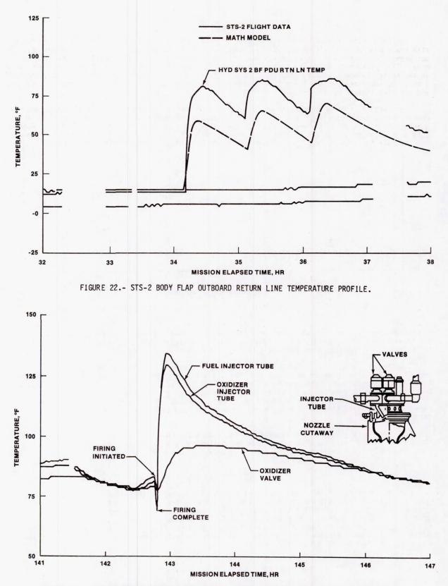
FIGURE 23.- STS-4 FORWARD PRIMARY RCS ENGINE TEMPERATURE RESPONSE TO 30-SECOND FIRING.
