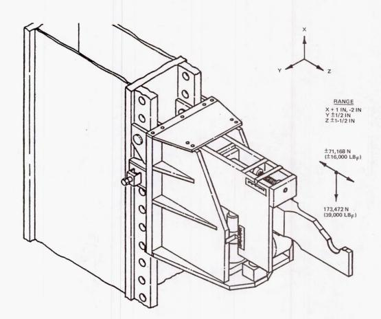
FIGURE 5. PRIMARY PAYLOAD SUPPORT FITTING MOUNTED TO SUPPORT BEAM
