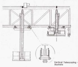
The design of the two bridges included provisions for support of the Zero- Gravity device used in opening and closing the payload doors.
