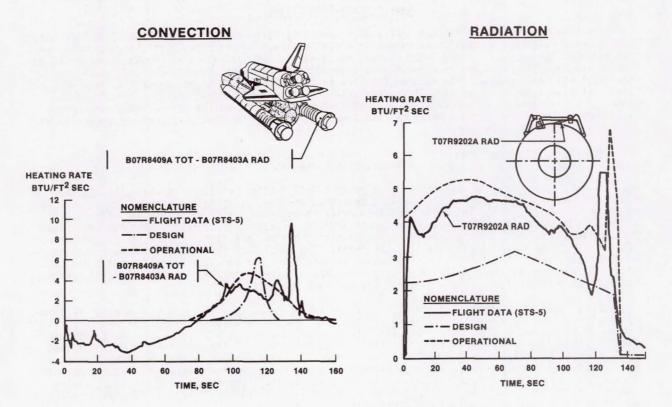
Shuttle flights STS-1 through 5. There was generally good agreement overall between flight data and preflight prediction. 17
