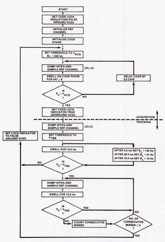
FIGURE 11.- SSP ACQUISITION-TRACKING ALGORITHM (S-BAND).
