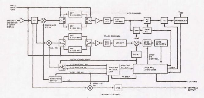
FIGURE 10.- S-BAND SPREAD SPECTRUM PROCESSOR (SSP) FUNCTIONAL DIAGRAM.
