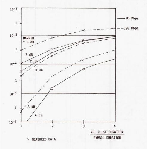
FIGURE 3: ILLUSTRATIVE IMPACT OF RFI PULSE DURATION ON SHUTTLE-TDRSS S-BAND RETURN LINK. (A  $\geq$  D  $\geq$  C  $\geq$  B)
