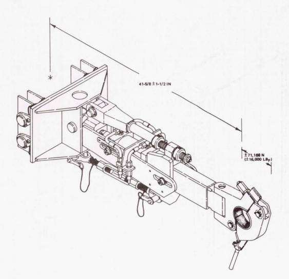
FIGURE 6. SECONDARY PAYLOAD SUPPORT FITTING MOUNTED TO SUPPORT BEAM
