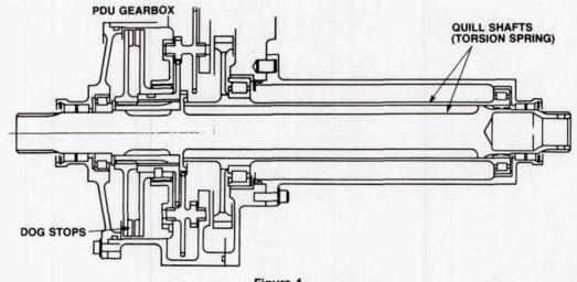
Figure 4 Quill Shaft and Dog Stops in PDU Gearbox
