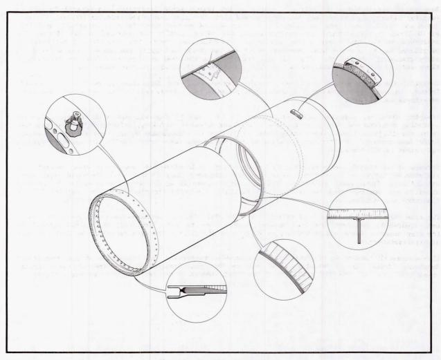
Figure 11 Arm Boom Construction
