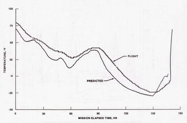
FIGURE 21.- STS-4 STARBOARD MAIN LANDING GEAR STRUT ACTUATOR TEMPERATURE PROFILE.
