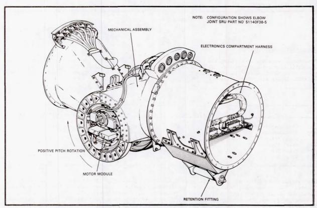
Figure 7 Overall Configuration of the Elbow Joint
