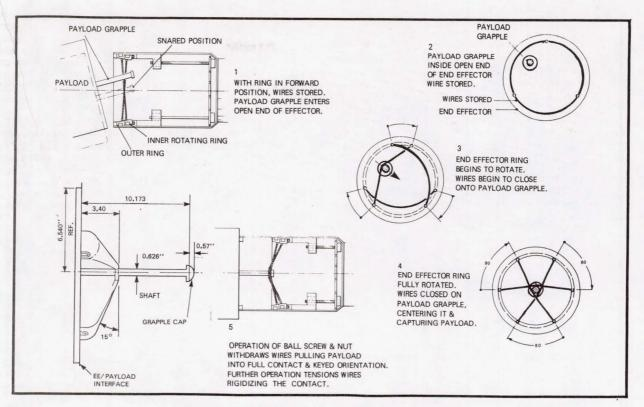
Figure 10 End Effector Capture and Rigidize Sequence
