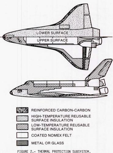
FIGURE 2.- THERMAL PROTECTION SUBSTSTEM.
