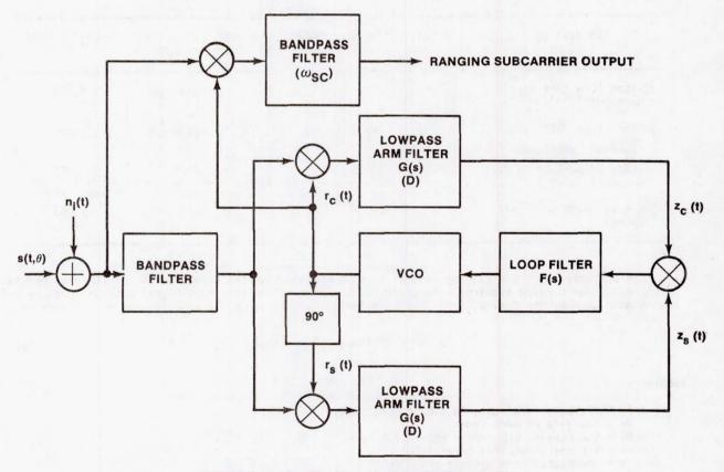
FIGURE 19.- COSTAS LOOP AND RANGING DEMODULATOR.
