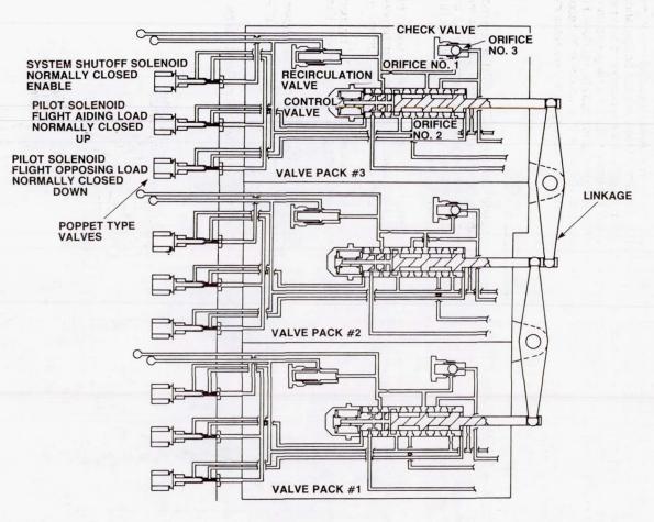
Figure 1A Body Flap Actuation Valve Pack
