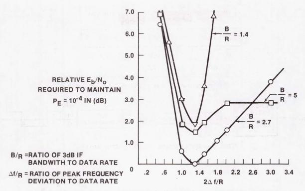
FIGURE 23.- RELATIVE BIT ERROR PERFORMANCE (BIPHASE DATA): DISCRIMINATOR DETECTION OF CONTINUOUS-PHASE FM MODULATION.
