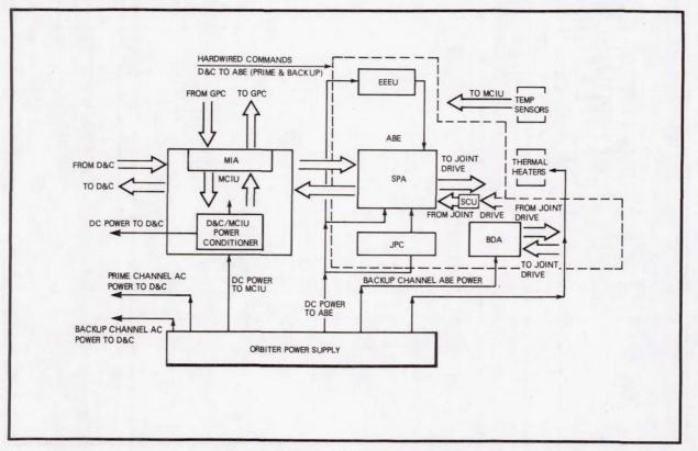
Figure 3 SRMS Electrical Subsystem Block Diagram
