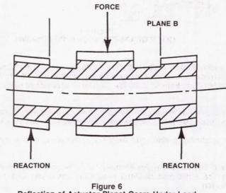
Deflection of Actuator Planet Gears Under Load
