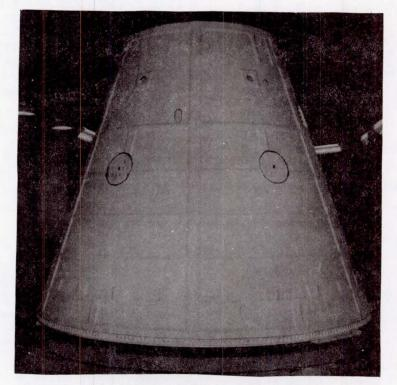
Figure 8. SRB Frustum with MSA-1 and Hypalon Paint Applied.
