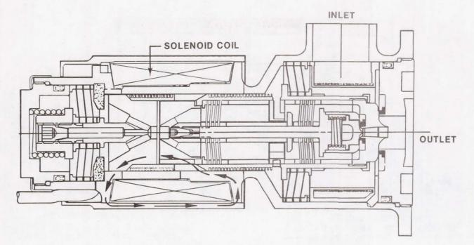
FIGURE 6.- CROSS SECTION OF PRIMARY THRUSTER VALVE.
